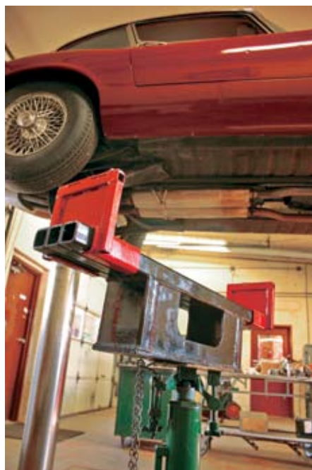
Stew has designed and built his own components to assist E-Type restorations, including two 360-degree body rotators and unique rear suspension supports for the two-post lifts.
