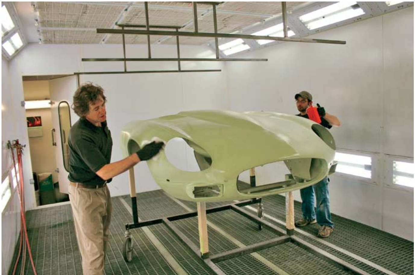
Working in the main shop's Accudraft downdraft spray booth, which has the capacity to change the air every 20 seconds, body and paint specialists Tom Jones and former fabricator Marc Rosenberg rub down a bonnet mounted on Stew's special 90-degree tiltable bonnet stand.
