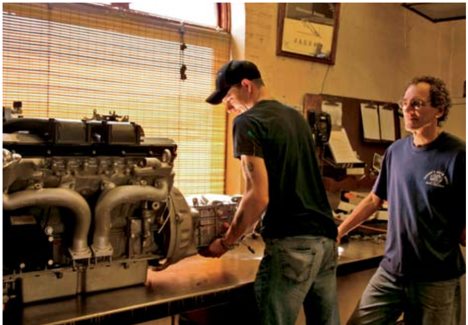
Mechanics Chris Stewart and Frank Marinelli mate a Borg-Warner T5 to a rebuilt V-12.
