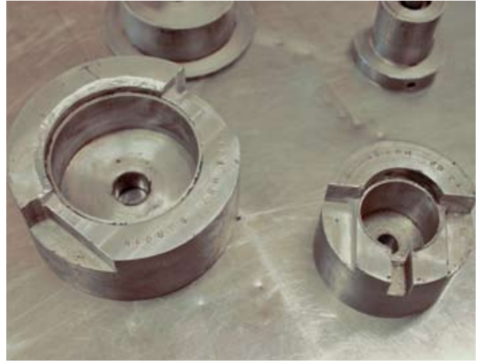
Years of specializing in E-Type restoration mean they've created devices like these machined aluminum radius arm bushing presses.
