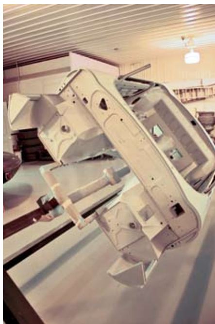
Stew has designed and built his own components to assist E-Type restorations, including two 360-degree body rotators and unique rear suspension supports for the two-post lifts.
